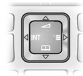
In the description below, the side of the control key (up, down, right, left) that you have to press in the different operating situations is marked in black, e.g.
