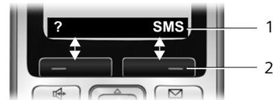
1 Current display key functions are shown in the bottom display line.
